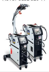
The AUTOPULSE 320-T3 is a 320 A, dual pulse MIG/MAG generator with 3 integrated motorised reels. It is an extremely advanced machine with 68 synergic curves for exceptional arc quality. Versatile, it can accommodate 3 different torches for welding steel, aluminium and brazing wire (CuSi3/CuAl8). The accessible interface and the quality of the wire feeders make welding on very thin sheet exceptional.
