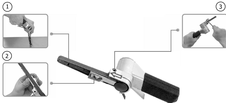
Press the side button and slightly press the end of the sander to reduce the belt tension. Remove the damaged belt and replace it with a new one:
