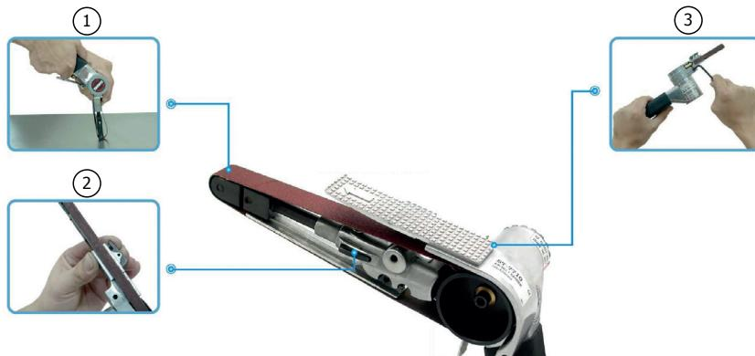
Press the side button and slightly press the end of the sander to reduce the belt tension. Remove the damaged belt and replace it with a new one:
