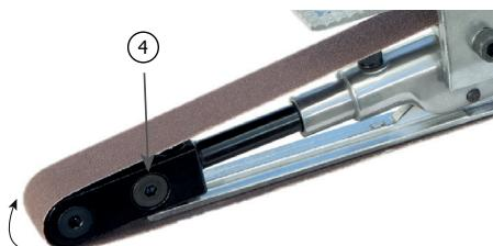
If the belt is not centered on the bracket, turn the screw ④ with a hexagonal wrench.
