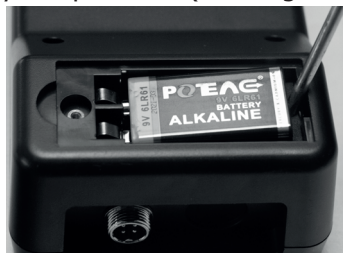
Remove the battery by levering it out with a screwdriver
